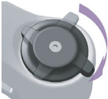
Figure 123: Changing compression adjuster to a harder setting
