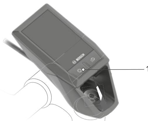
Figure 113: Position of On-Off button (on-board computer)
