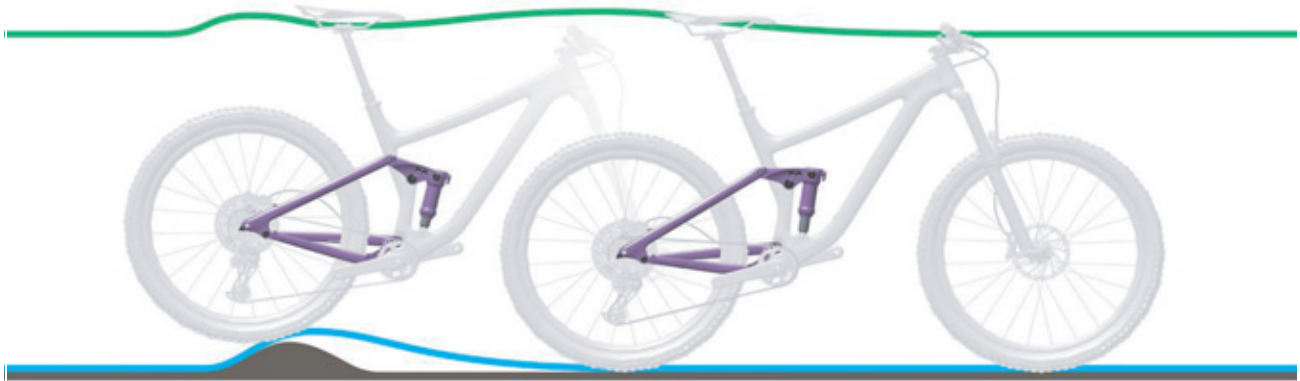
Figure 148: Excessively hard damping in the rear frame damper on bumps
