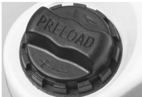
Figure 79: Sag setting wheel on the suspension fork crown
