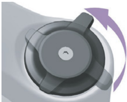
Figure 124: Changing compression adjuster to a softer setting
