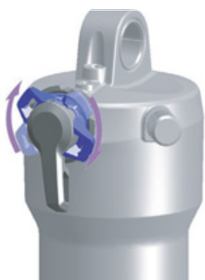
Figure 147: Changing compression adjuster to a harder setting
