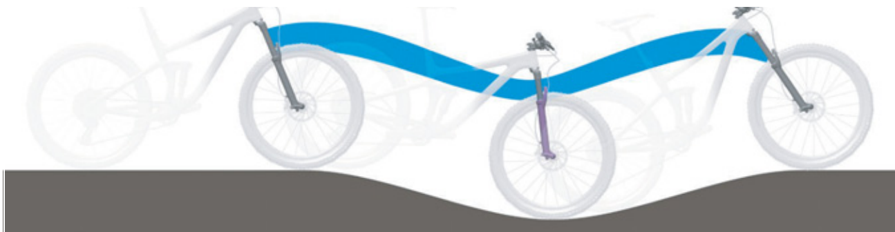
Figure 6: Optimum fork riding performance on hilly terrain
