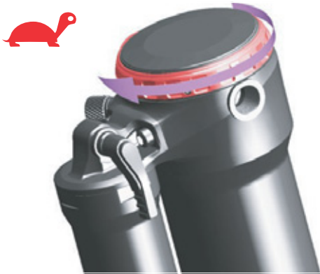
Figure 143: Turning rebound damper towards tortoise symbol
