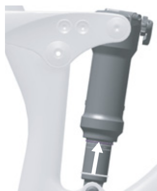
Figure 87: Moving the O-ring on the rear frame damper
