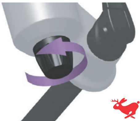
Figure 137: Turning rebound damper towards hare symbol
