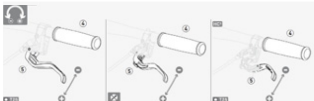
Figure 77: Adjusting the grip distance on a Magura disc brake lever
