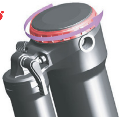
Figure 145: Turning rebound damper towards hare symbol
