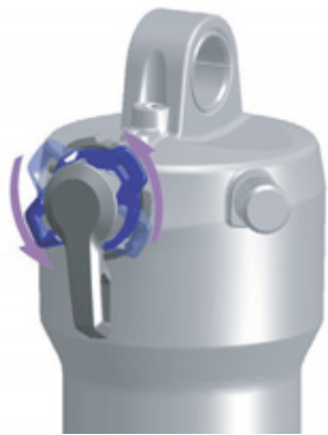
Figure 149: Changing compression adjuster to a softer setting
