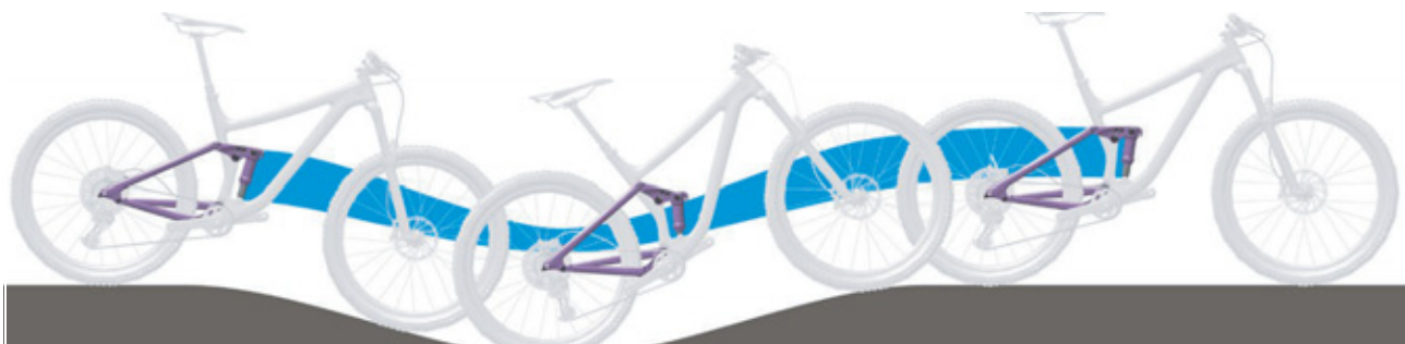
Figure 146: Excessively soft suspension in the rear frame damper on hilly terrain
