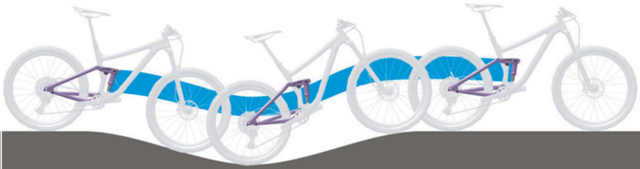
Figure 97: Optimum rear frame damper riding performance on hilly terrain
