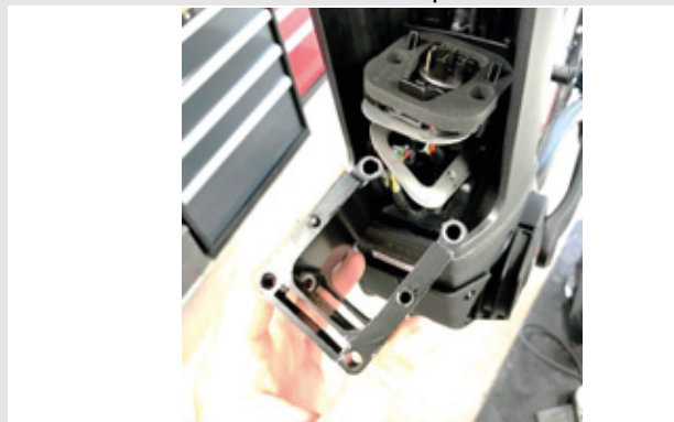
Figure 38: Pulling out the PowerTube adapter
