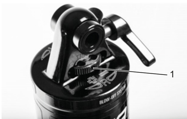
Figure 91: Suntour rebound adjuster wheel (1) on the rear frame damper
