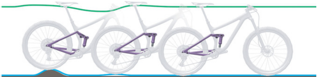
Figure 142: Rear frame damper rebounding too quickly
