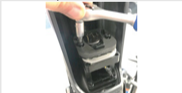
Figure 35: Undoing screws on battery mount
