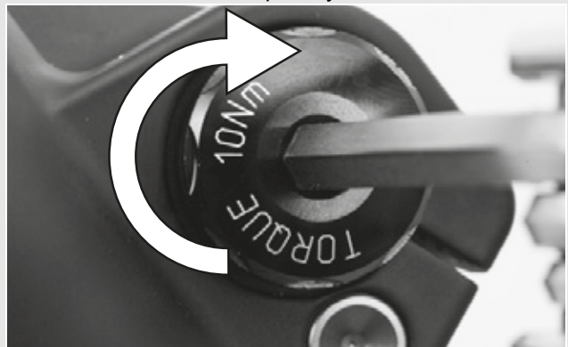
Figure 52: Tightening the inserted axle
