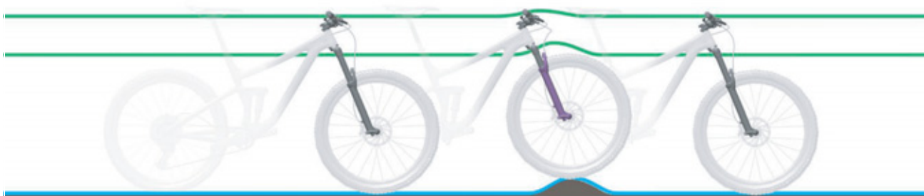
Figure 7: Optimum fork riding performance over bumps
