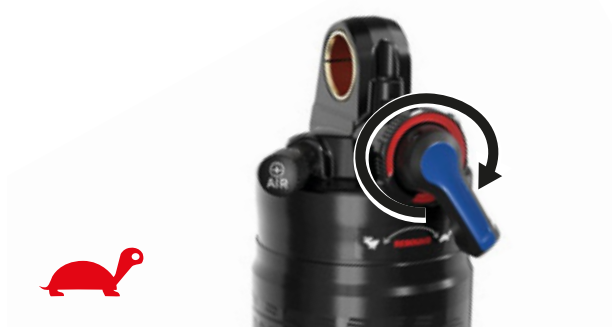
Figure 95: Reducing the rebound speed
