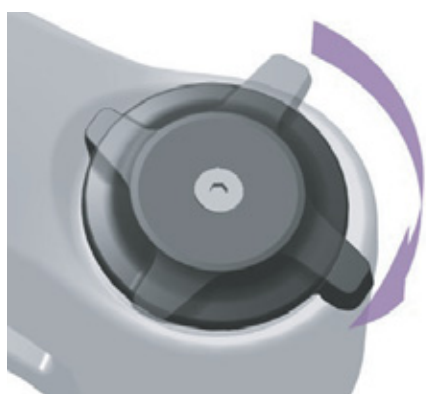
Figure 139: Changing compression adjuster to a harder setting
