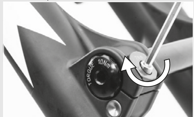
Figure 53: Tightening the securing clip
