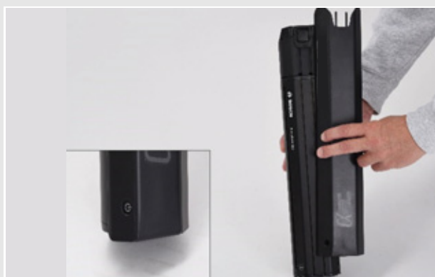
Figure 47: Pushing the battery cover onto battery
