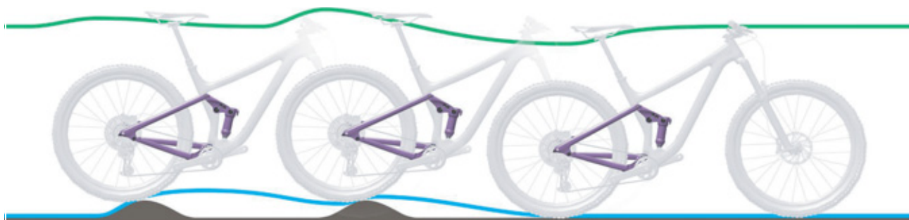
Figure 144: Rear frame damper rebounding too slowly
