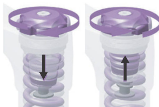
Figure 82: Screwing and unscrewing the pre-tension adjustment ring.
