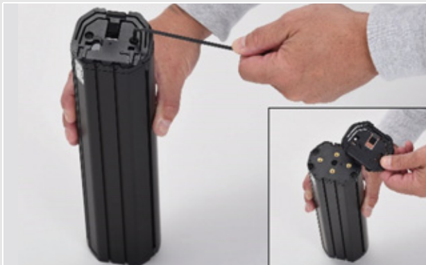
Figure 41: Detaching the upper interface
