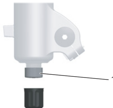
Figure 92: FOX rebound adjuster (1) on the fork end
